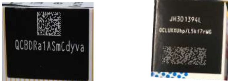
Fig. 33a) ISO/IEC 16022 Data Matrix with Tobacco data Source: E.D.C. Fig. 33b) AIM DotCode placed on unit level package source: Incert
