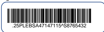
Figure 29) - Example Code 128 with two ASC DI headed data elements concatenated by separator “^”
